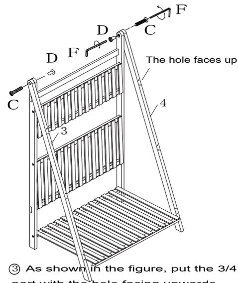
③ As shown in the figure, put the 3/4 part with the hole facing upwards and the big hole facing outwards, and assemble it with hardware C.D.
