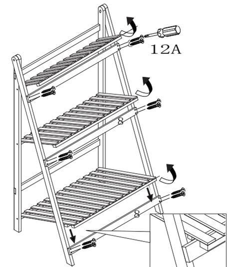
④ Turn part 5/6/7 upside down and assemble part 8 with hardware A as shown. Note that, clamp board 7 to part 8 as the arrow.
