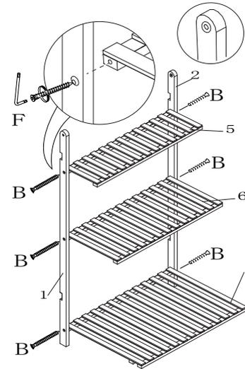
① As shown in the figure, the opening of part 1/2 is facing backward, and the board 5/6/7 is assembled with hardware B.
