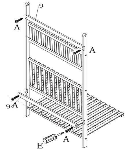
② Insert part 9 into the opening as shown in the figure, and assemble it with hardware A.
