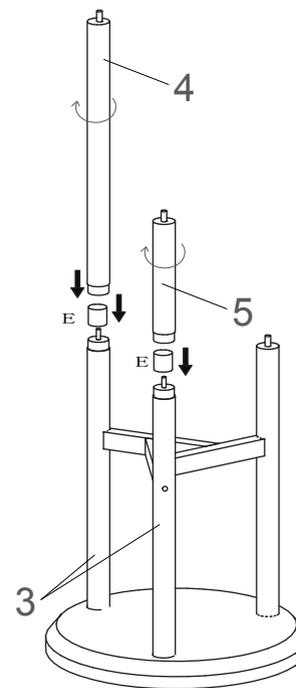
3. Connect parts (4)/(5) through sleeve E to lower support bar (3)
