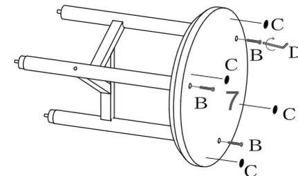
2. Connect the part (7) with the support bar with the hex self-tapping screw B, then put the foot pad on C.
