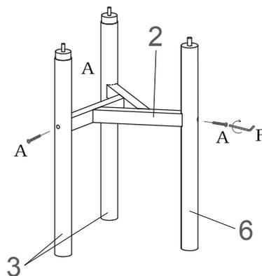
1. Connect part (3)/(6) to part (2) with the hex self-tapping screw A.
