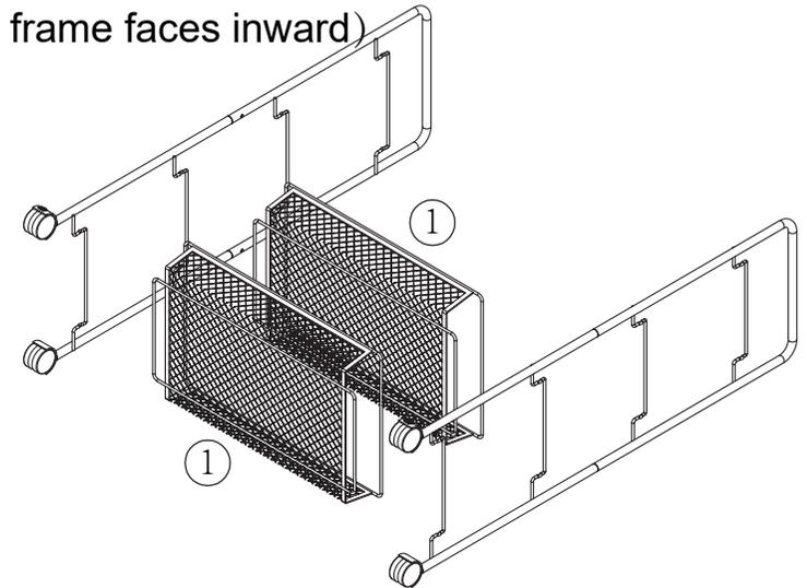
Straighten the rack and install the rest of the baskets in turn.
